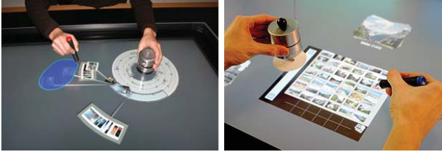
Fig. 4. Left: Organizing images into events with PhotoHelix. Right: Scrolling and zooming images with the help of PhotoLens [7].
