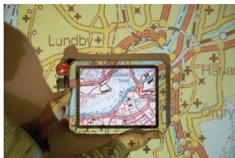
Fig. 1. Occlusion and seamless integration using front projection [61].
