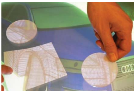
Fig. 5. Beyond-the-surface projection with a switchable diffuser [26].
