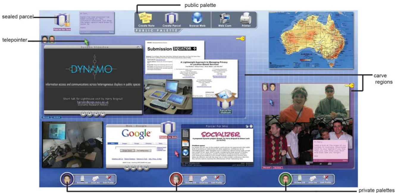
Fig. 4. Dynamo interface with a selection of media, two carve regions, three personal palettes and a public palette [15]
