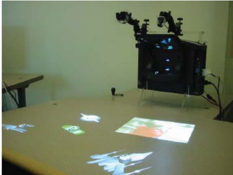
Fig. 2. Avoidance of occlusion by using a mobile projector [75].
