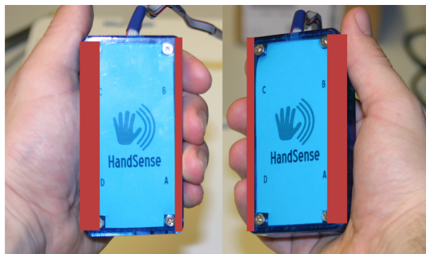
Figure 1. HandSense is able to determine whether a device is held in the left or right hand by measuring the capacitance to each side. As the ball of the thumb is thicker than the fingers, it causes higher sensor readings.
