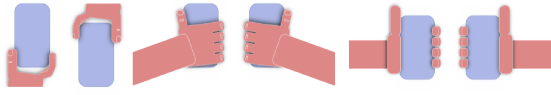
Figure 2. HandSense can distinguish six different ways of grasping a device. From left to right: hold up, pull out, grasp right, grasp left, hold left, hold right.
